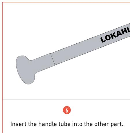
*Make sure that the front (flat) side of the handle is perfectly parallel to the front side of the blade.*
